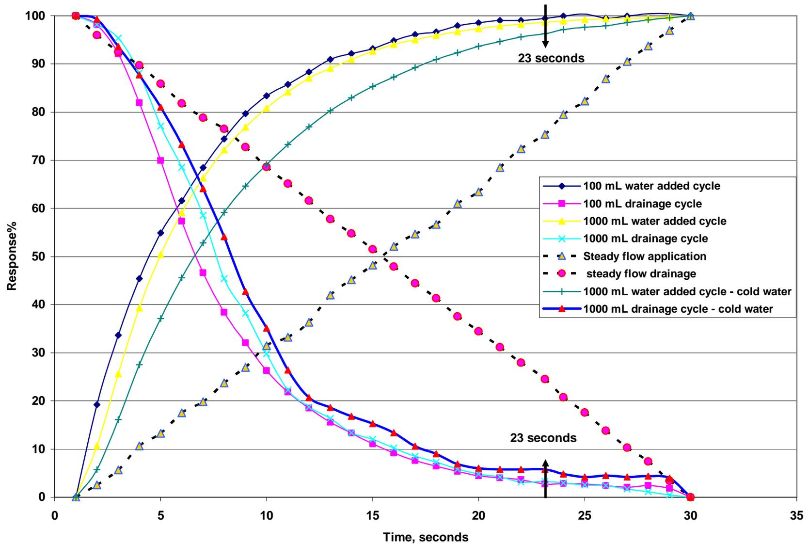
Figure 10: Effect of the amount of water applied, flow type, and water temperature on PT300-Medical sensor’s performance response%.
