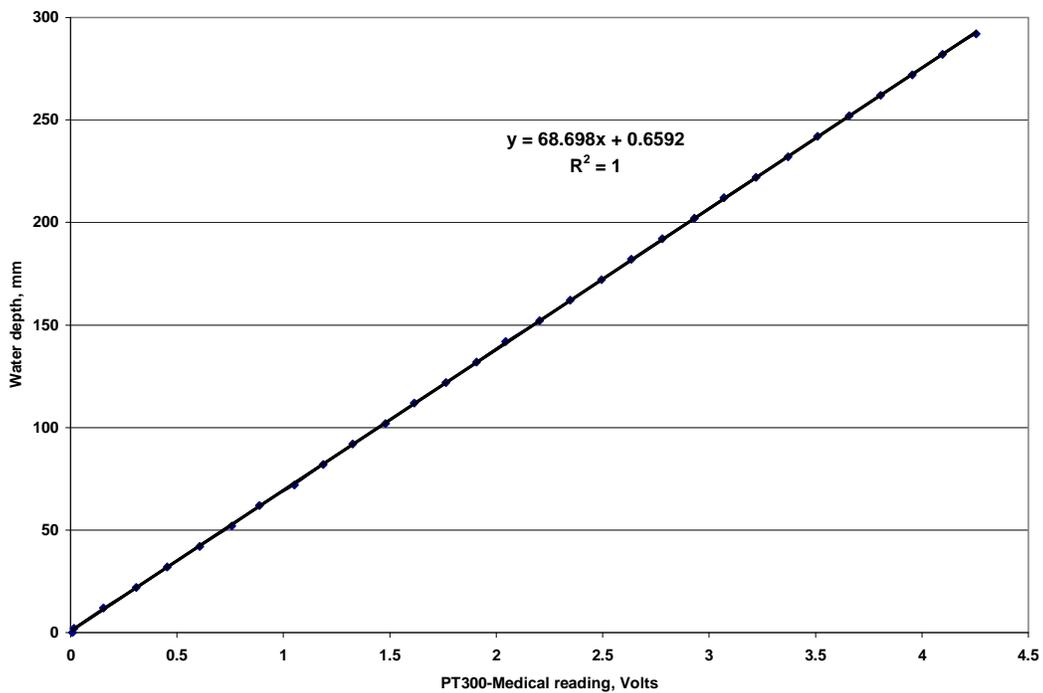
**Figure 8: Linear fitted extrapolation between PT300-Medical readings and measured water depth in the reservoir when 100 mL water is drained from system at each time step.**
