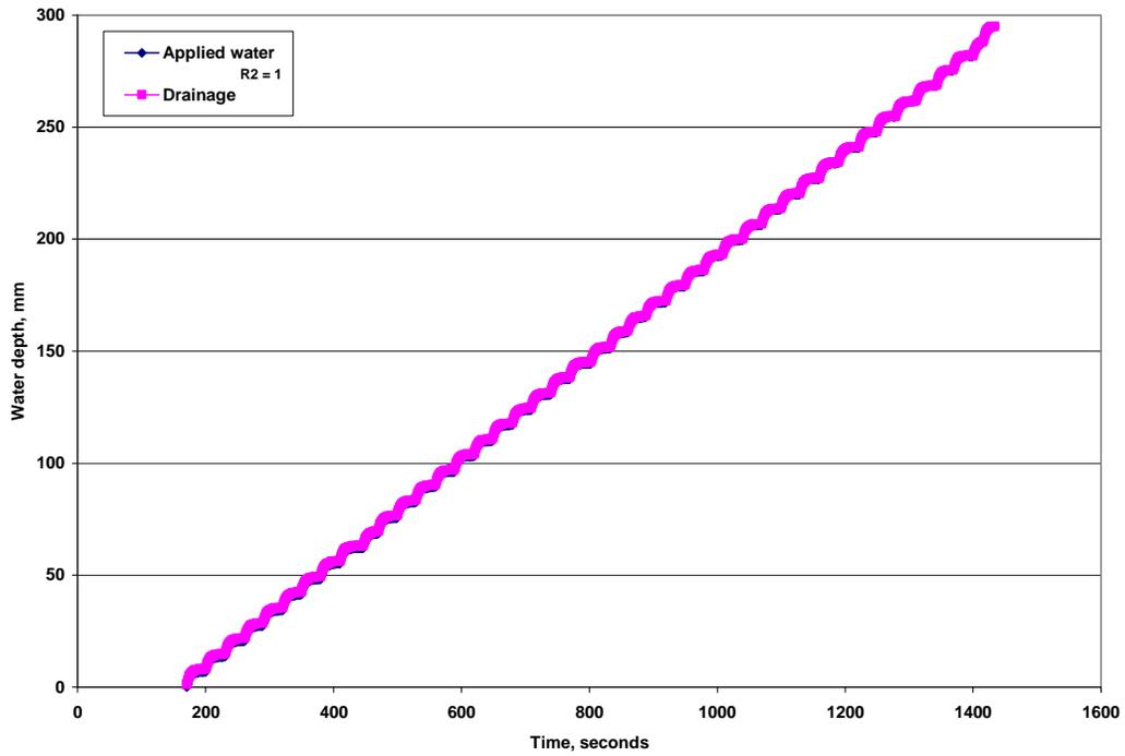
**Figure 9: Lag time between applied water and drainage cycles for the PT300-Medical where a volume of 100 mL water is applied or drained from the system at each time step.**
