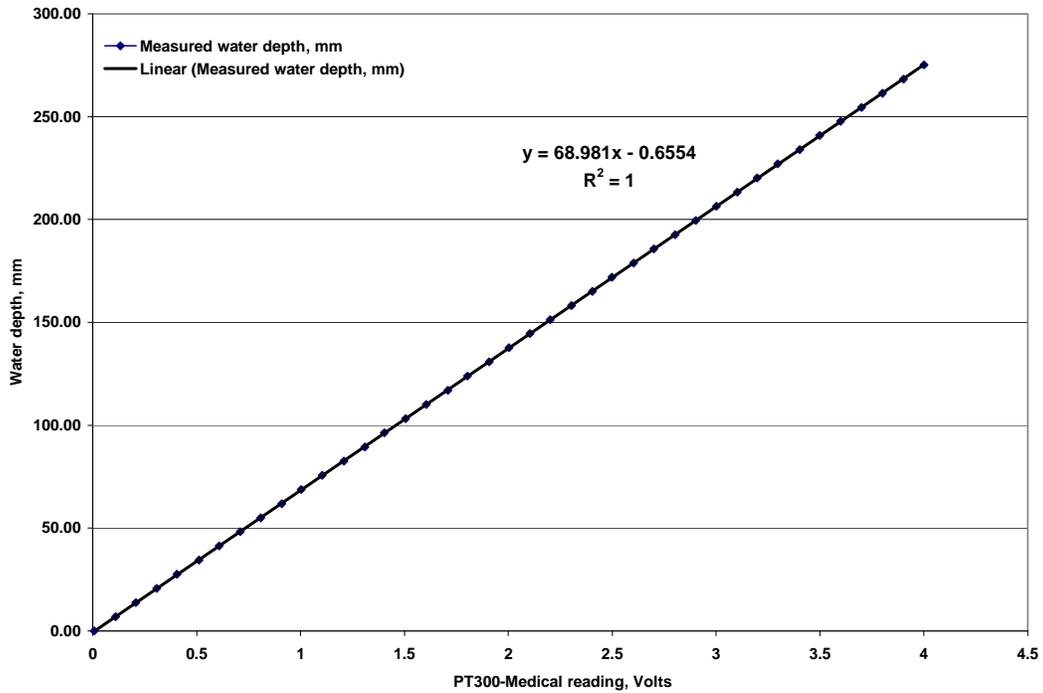
**Figure 7: Linear fitted extrapolation between PT300-Medical readings and measured water depth in the reservoir when 100 mL water is applied to the system at each time step.**
