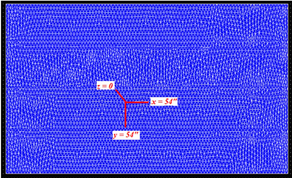
**Figure 2: Finite element geometrical mesh for the mesocosm soil domain.**
