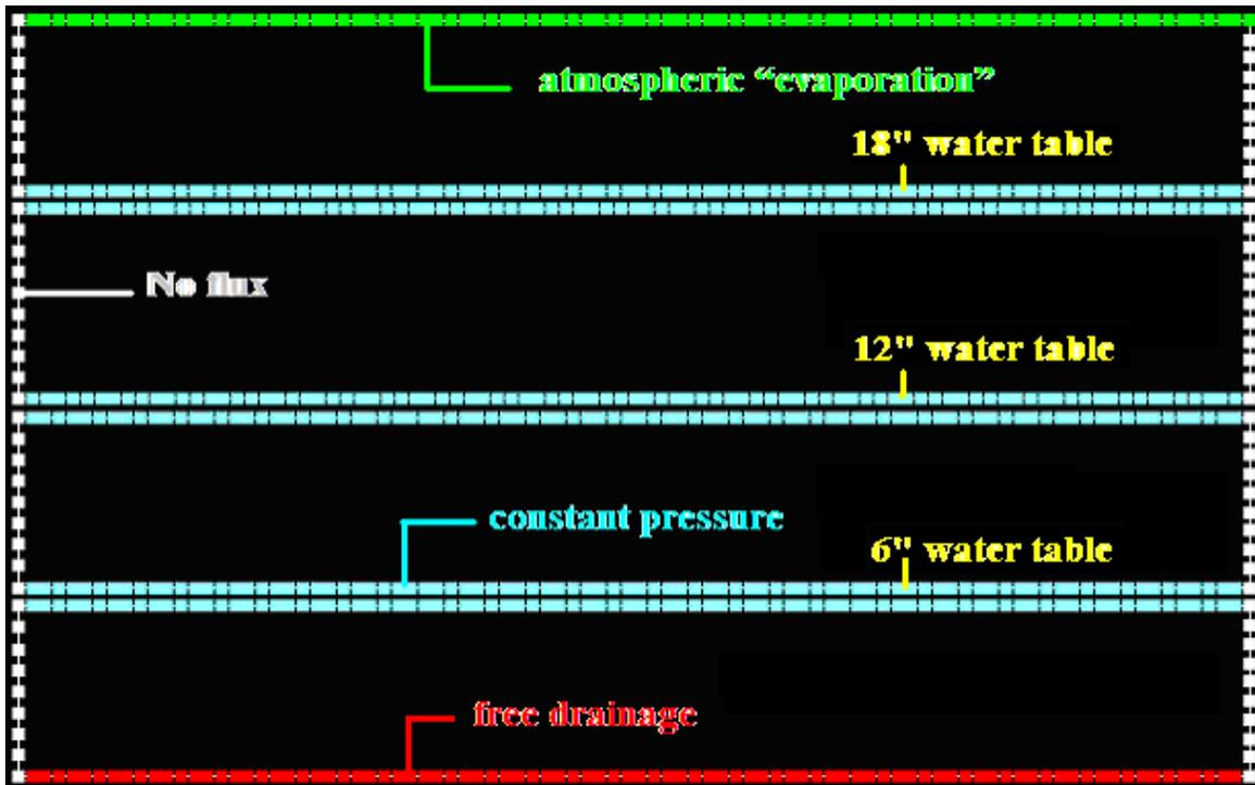
Figure 4: Boundary conditions selected for the mesocosm soil domain
