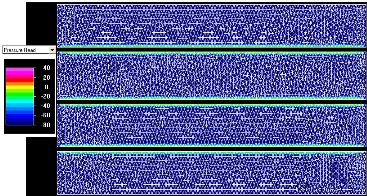
**Figure 5: Soil water potential distribution along the mesocosm soil domain.**
