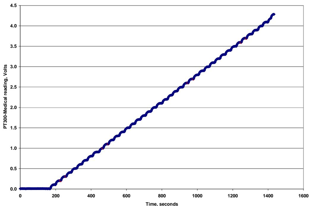
**Figure 6: Performance of PT300-Medical as a function of hydrostatic pressure changes when 100 mL water is applied to the system at each time step. Time difference between the red points represents the time cycle of the response % in Table 2.**
