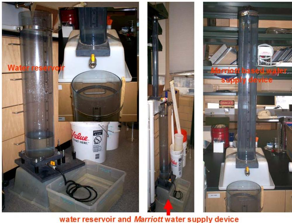
Figure 1: Water reservoir and Marriott based water supply device for testing the prototypes.
