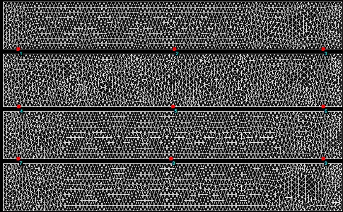
Figure 3: Distribution of the observation nodes (corresponding to tensiometers and TDRs locations at 6, 12, and 18 inches) along the mesocosm soil domain.
