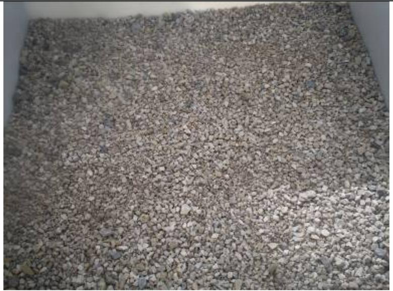
**4- Sand filter pack around the screened wells and the piezometers.**
