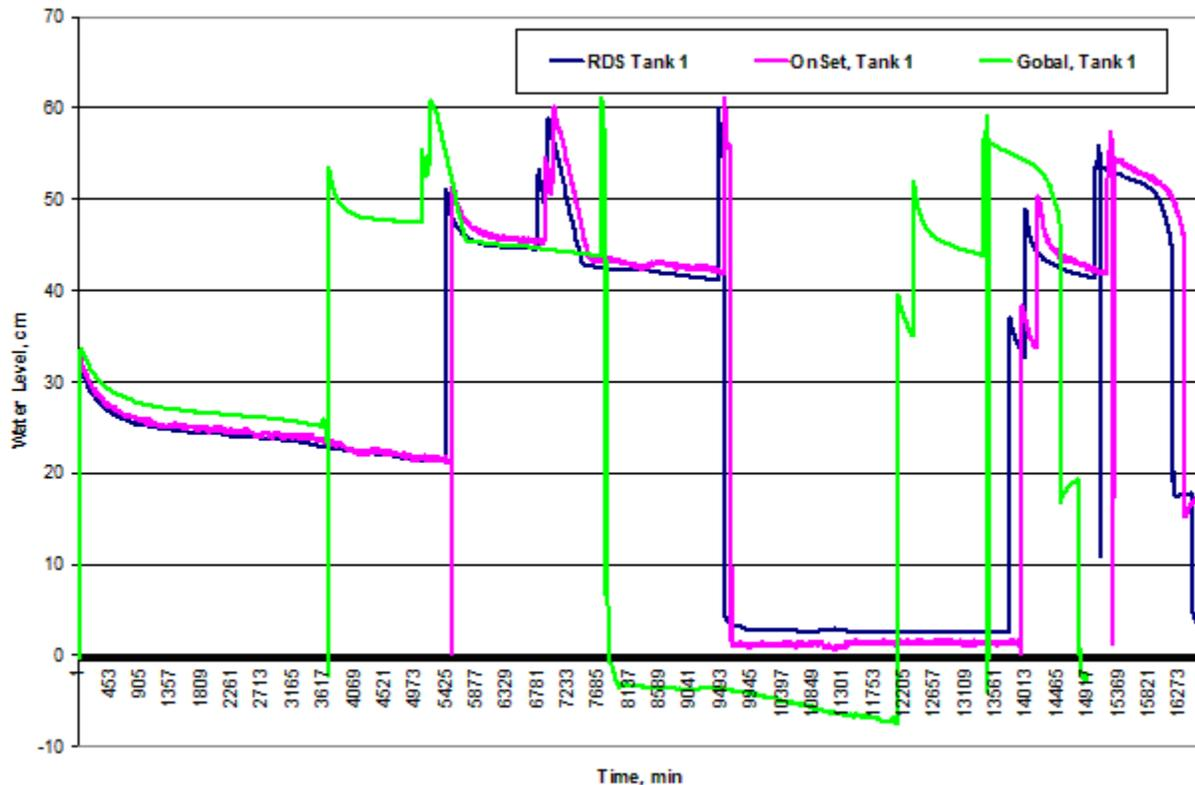
**Figure 3: Evaluation of selected water level sensors performance during two consecutive wet-dry cycles in a mesocosm.**
