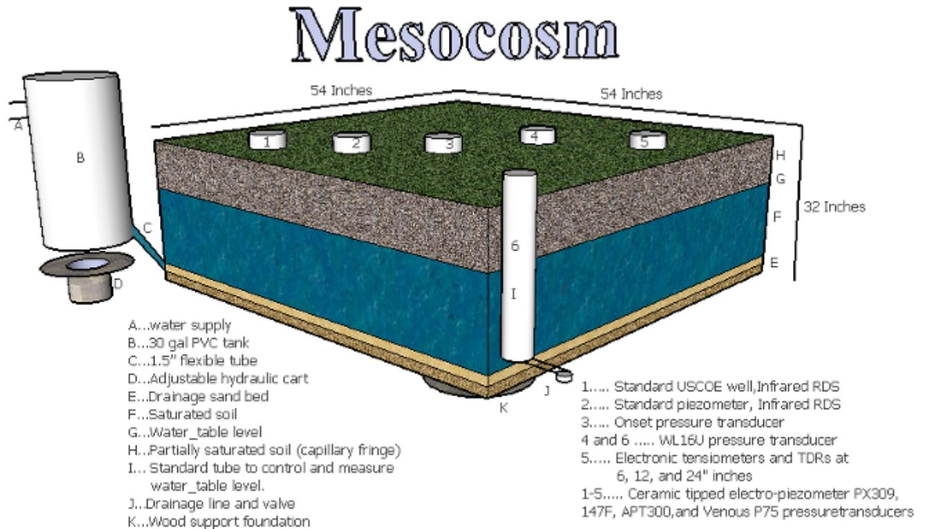
**Figure 2: Schematic diagram and basic description of the different soil/water level sensors for the water level mesocosms at Virginia Tech greenhouse.**
