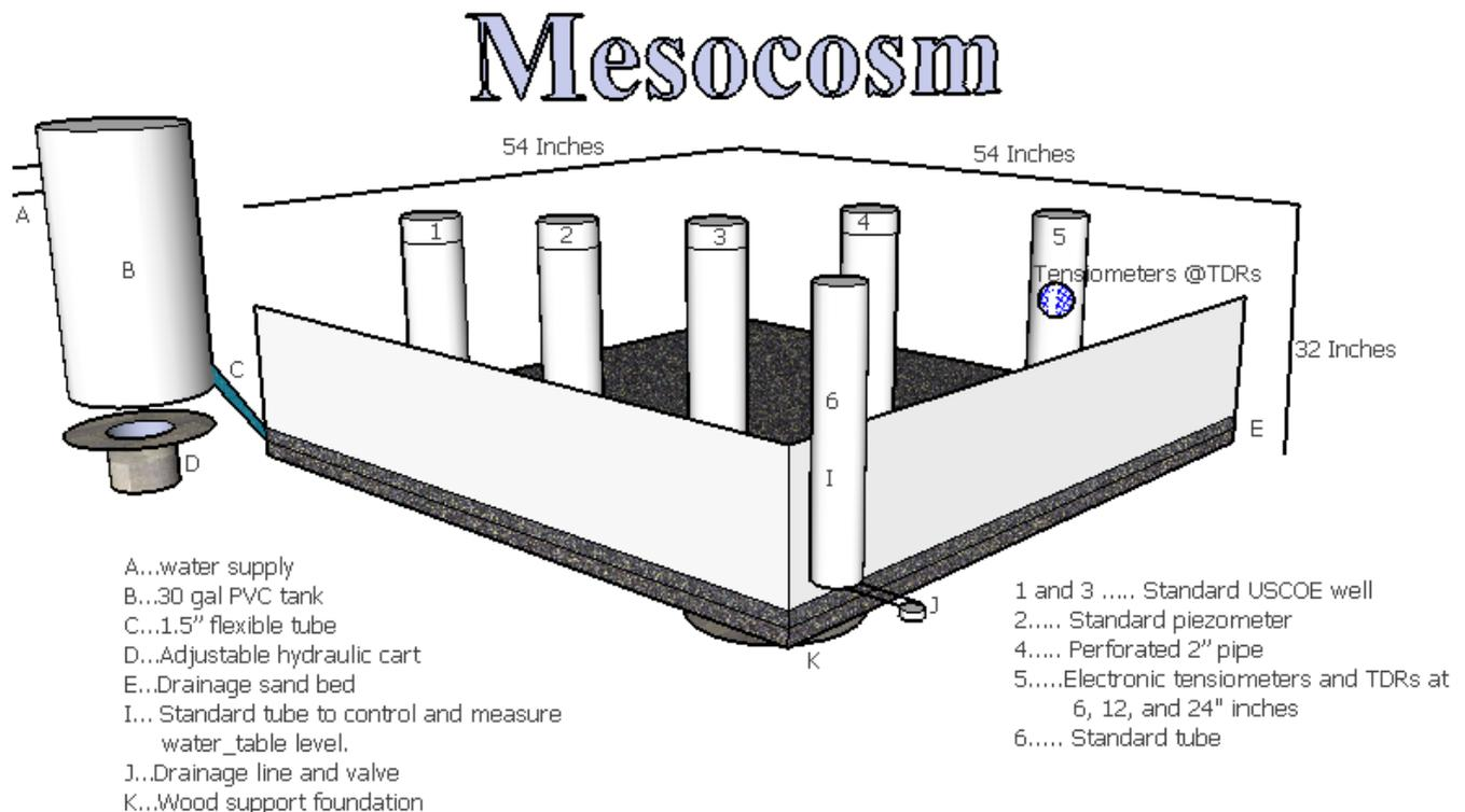
**Figure 1: Schematic diagram of the water supply line, drainage system, wells and piezometer distributions for the water level mesocosms at the Virginia Tech greenhouse facility.**
